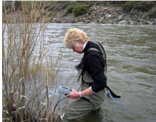
Jane Tollett of GCWIN collects river and stream water quality data with a YSI sonde. All data is shared in a public database called WILBUR.
